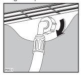
Always use the hose supplied with the appliance. The inlet hose must not be lengthened.
